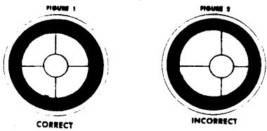
Figure 2 indicates main mirror out of adjustment.
