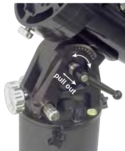
ALTITUDE LOCK LEVER Operation
