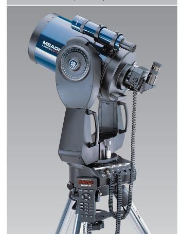
**Precision GPS Alignment:** Telescope alignment is accomplished *automatically* using signals from the Global Positioning System (GPS), a satellite system that enables extremely precise communication to the telescope of the observer's latitude and longitude, as well as local time. Integrated true-level and North electronic sensors in combination with a 16-channel GPS receiver located in the
