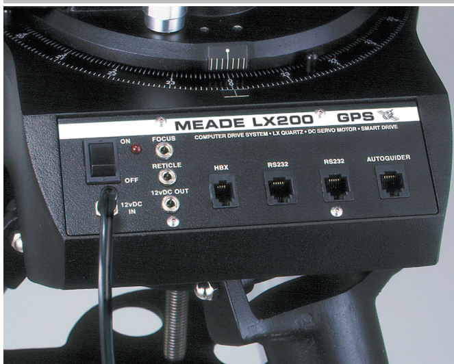
Control panel of Meade 7", 8", 10", and 12" LX200GPS models.
